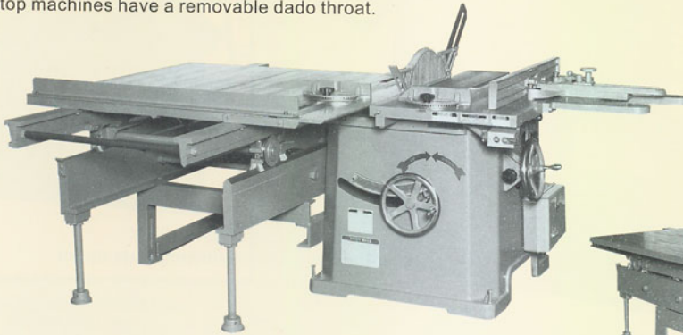
Northfield #4 Tilting Arbor Variety Saw with standard rolling table, 24" extended table to right, and Micrometer Adjust Fence.
