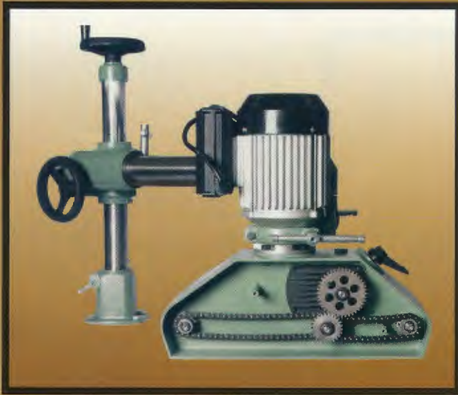
REAR VIEW SHOWING ROLLER FEED CHAINS AND STUD GEARS
