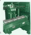
jointed for concentricity and hollow ground with a motor/diamond wheel assembly provided with the 360. Cutterhead maintenance takes less than three hours. High impact grinding shield provided.
