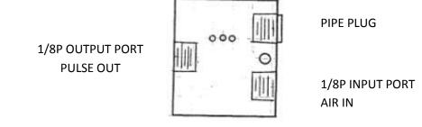
If the output port delivers no air -the valve is bad. If the output port flows air continuously the valve is bad. If the output port leaks a small amount of air after the initial pulse the valve is bad.
