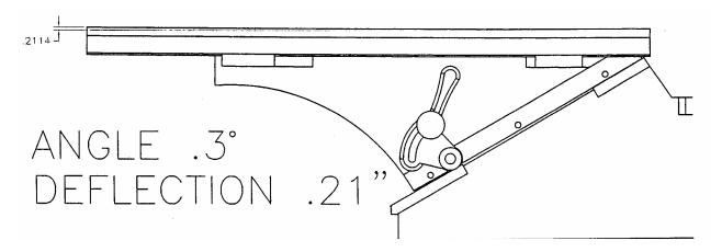
When a piece of stock was edge jointed with the out feed table in this "down" position, a convex cut was generated allowing the formation of a spring joint.
