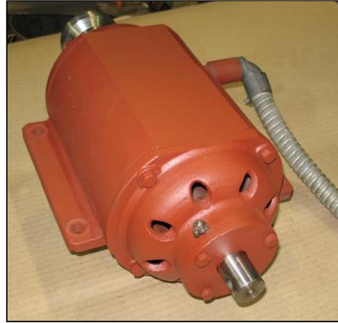
Open style Arbor Motor used on Table Saws from 1931 – 1957
