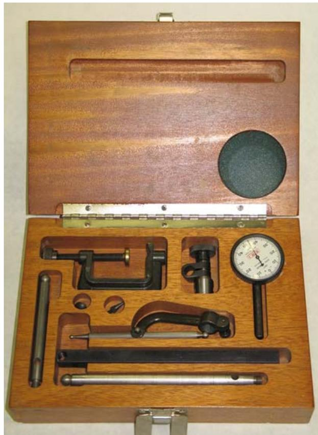
This is the indicator set that is used to establish the horizontal alignment of the grinder rail to knife slot.
