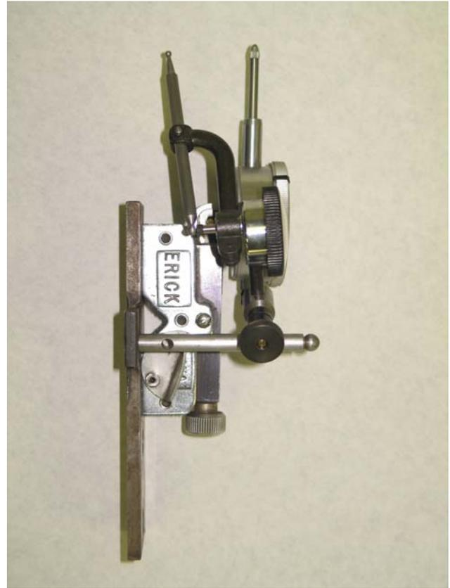
These pictures show both indicators in position on the mount plate. The large indicator checks the vertical alignment. The small indicator checks the horizontal alignment.
