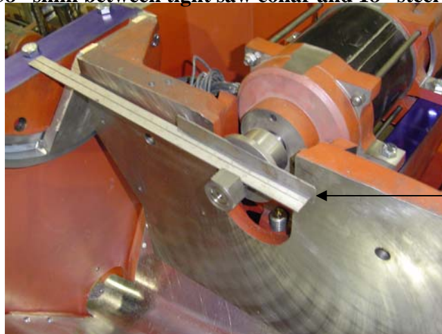
.0938" shim between tight saw collar and 18" steel rule
