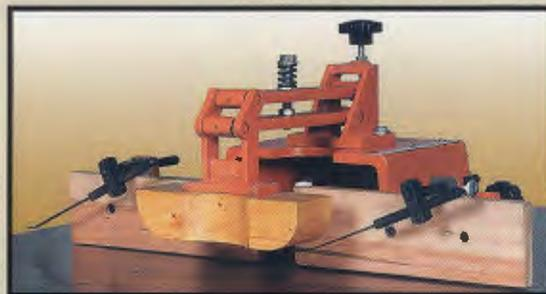
**BASE:** Heavy one piece casting with flanged floor base gives firm setting. Yoke ways are carefully machined to assure full yoke bearing.
