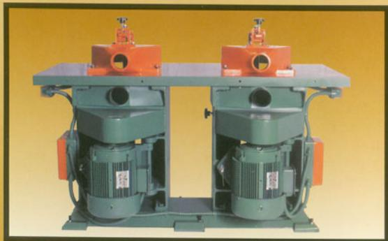
Rear view showing sub table dust outlets and guard mounting. Drive motors are mounted on hinged motor base. Gives accurate belt tension. Pulleys and belts are guarded.
