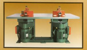
Rear view showing sub table dust outlets and guard mounting. Drive motors are mounted on hinged motor base. Gives accurate belt tension. Pulleys and belts are guarded.
