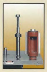
The spindles are machined from stressproof steel and are precision ground. The wide separation between the upper & lower sealed for life bearings provides extreme shaft rigidity when running large diameter cutterheads. The heavy yoke assembly with full length gibbed vee ways maintains deflection-free bearing and spindle alignments.
