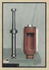
The spindle is machined from stressproof steel and is precision ground. The wide separation between the upper & lower sealed for life bearings provides extreme shaft rigidity when running large diameter cutterheads. The heavy yoke assembly with full length gibbed vee ways maintains deflection free bearing and spindle alignments.
