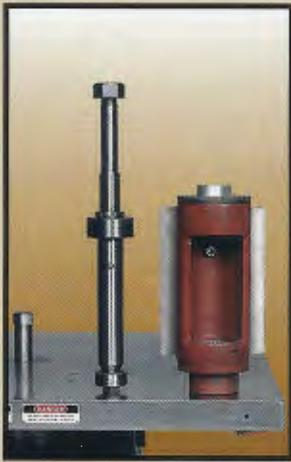
The spindle is machined from stressproof steel and is precision ground. The wide separation between the upper & lower sealed for life bearings provides extreme shaft rigidity when running large diameter cutterheads. The heavy yoke assembly with full length gibbed vee ways maintains deflection free bearing and spindle alignments.
