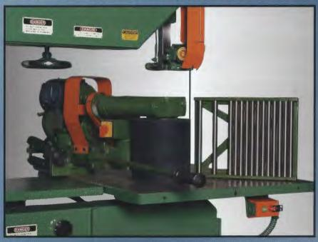
Detail of Roller Fence and rubber covered feed drum.
