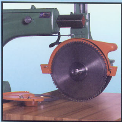
Photo shows the guard removed for blade changing
